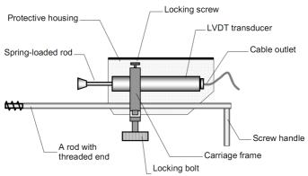
The probe is connected by a standard 1-meter cable to the waterproof box with the signal conditioner inside. A signal conditioner provides excitation of the LVDT and production of standard linear output signal. The output cable length should be specified in the order if required.
