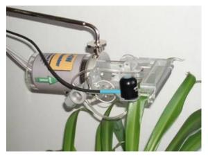
The LC-4W Leaf Chamber has a special plate for mounting optional Quantum sensor for measuring Photosynthetic Photon Flux (PPF) in  $\mu$ mol·m-2·s-1, if necessary.
