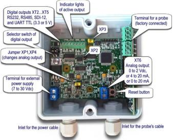
Connect according to the desired output:
