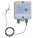
in diameter. Small size of the probe and its special design provide almost negligible disturbance of the natural leaf temperature.
