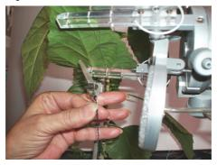
2. Mount the LT-LC sensor on a lower part of a plastic clip between the first and second clamping threads. You may use any of the paired clips.
