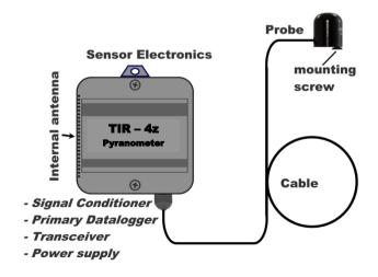
The probe is connected by a standard 3 meter cable to the waterproof box with electronics, which combines signal conditioner, primary datalogger, RF 2.4 GHz transceiver, and power supply (3xAA Alkaline batteries).
